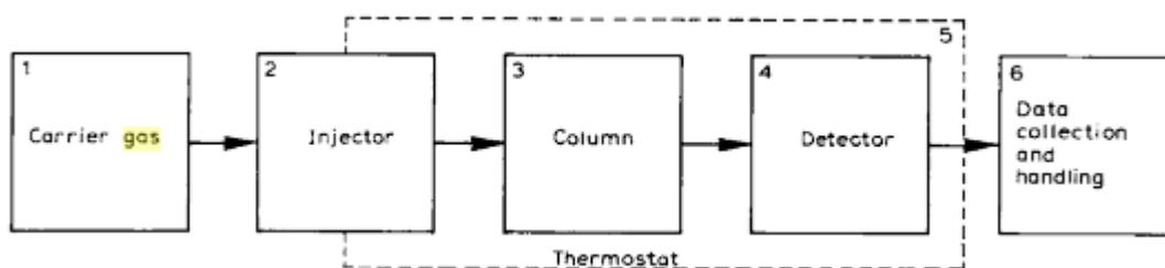
Figure 1: Schematic description of gas chromatography
